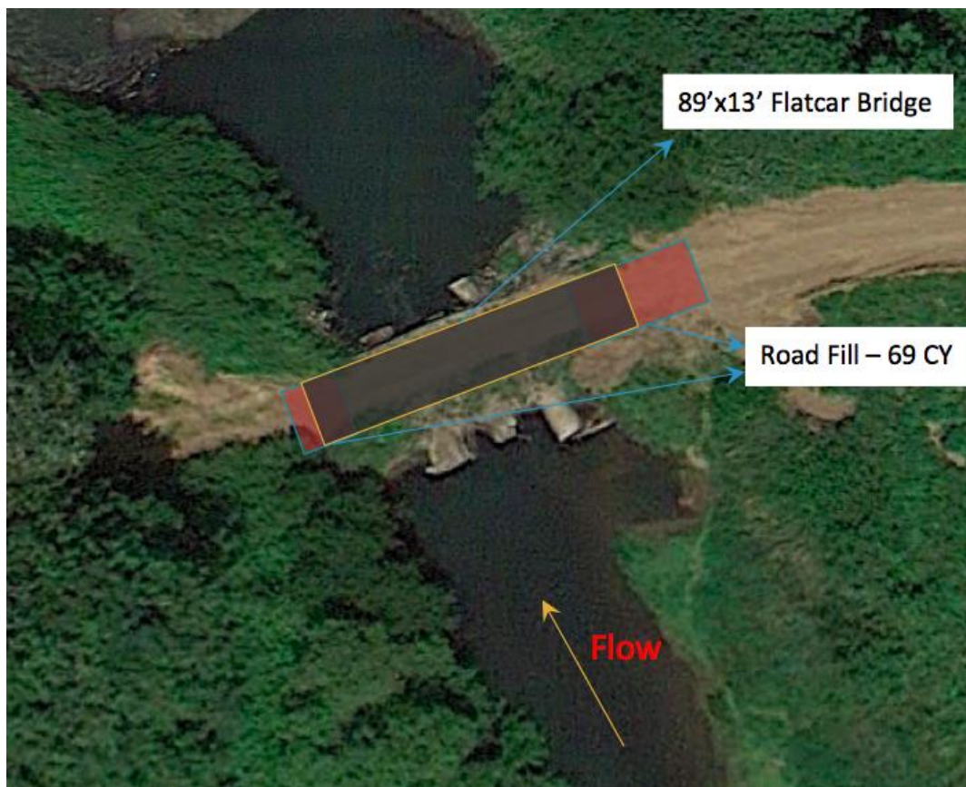
Figure 7 The above picture is a satellite photo with a plan view of the proposed design overlaid on it. The grey box represents the steel flatcar and the red represents backfill.
