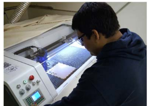
OPeNS Lab Technician, Manuel Lopez, makes adjustments to the laser cutter which will translate into a cut design. The possibilities are endless as the laser can cut through almost any material someone would like to work with.
