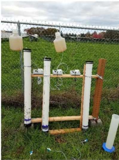
Column reactor set-up at the field site
