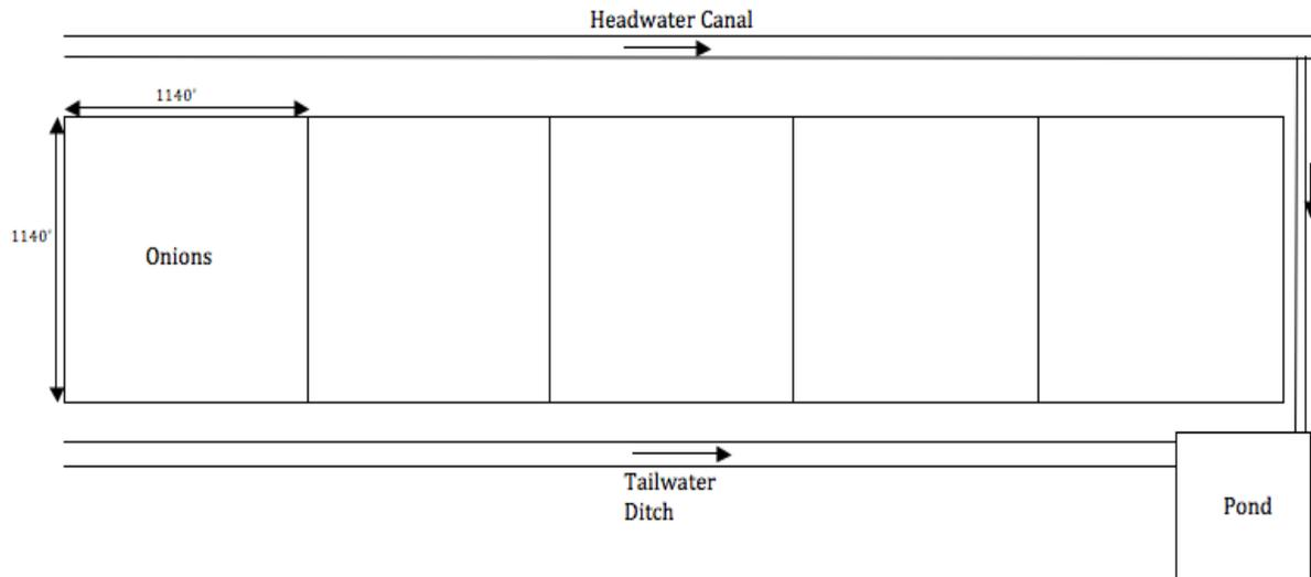
**Figure 3. Schematic of field layout with filtration pond and tailwater collection (not to scale)**
