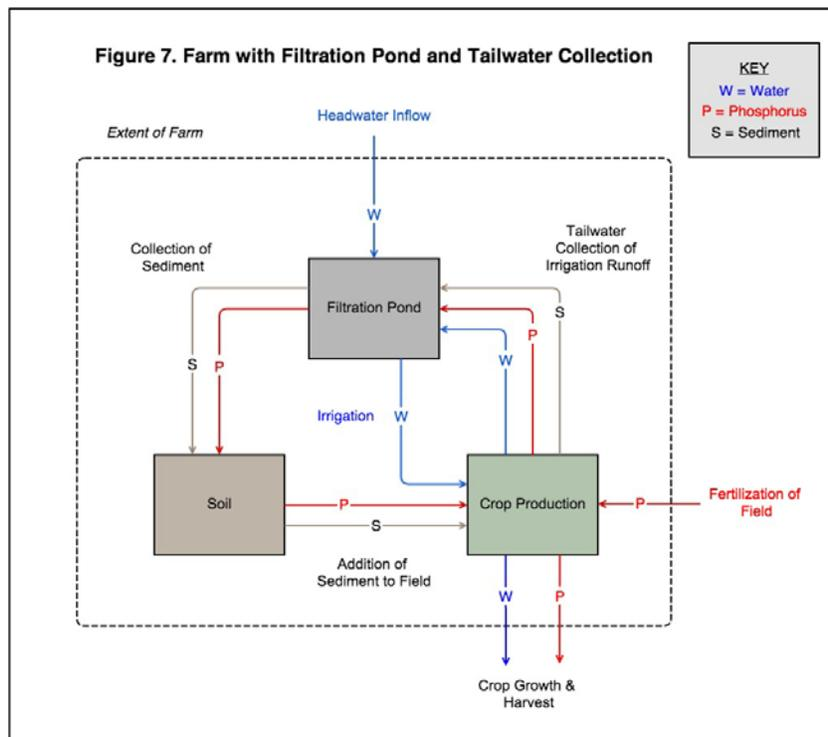
Figure 7. Systems diagram of a farm with a pond and tailwater collection
