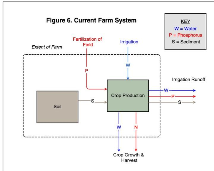
Figure 6. Systems diagram of a farm without a pond or tailwater collection
