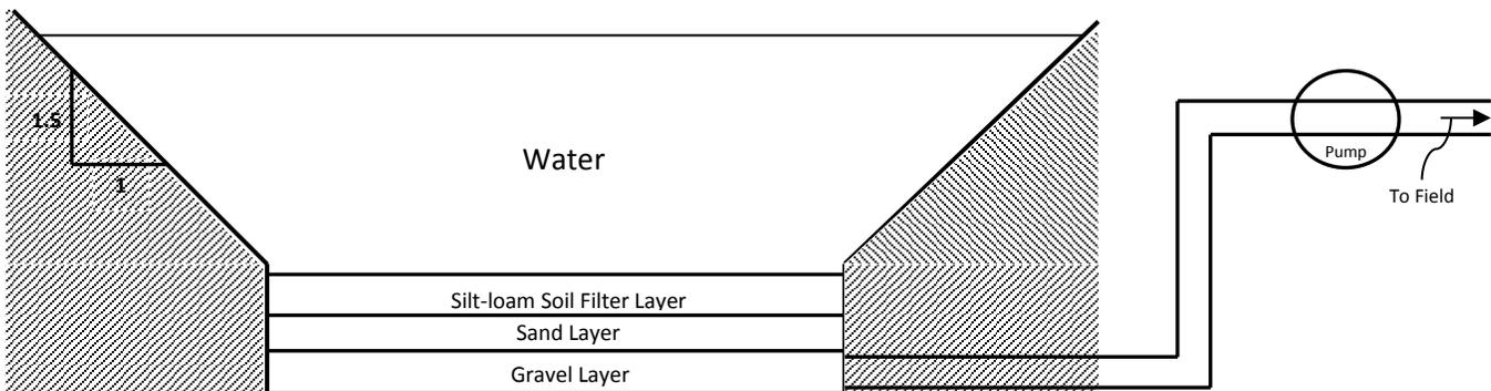
**Figure 4 Filtration pond cross-section with gravel, sand, and soil media layers (not to scale).**
