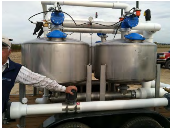
Figure 5: The sand media filtration system used in drip irrigation. This equipment is sold by Clearwater Supply locally in Malheur County.
