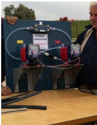
Figure 3: The chlorine dioxide generation system sold by CH20.
