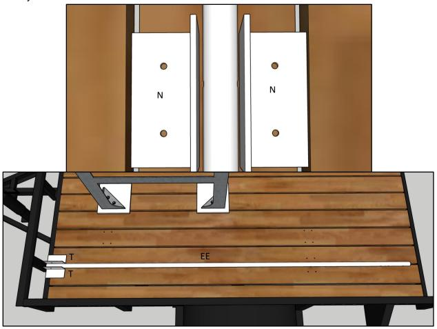
$\underline{\text{Step 8.3}}$  – Fit the hardware that secures the outer antenna pole to the angle irons that make up the base of the antenna mount.
